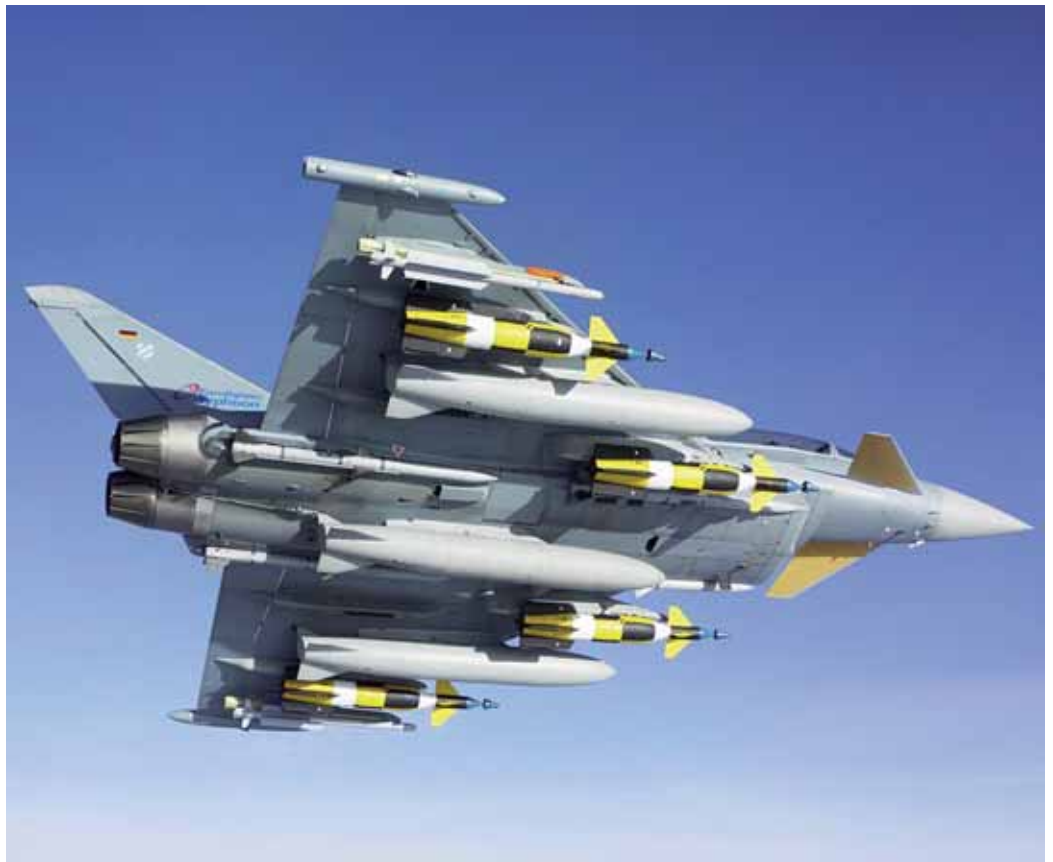
EUROFIGHTER IPA 3 in a Test Flight with 4 x Paveway II, 4 x AMRAAM Air-to-Air Guided Missiles, 2 x IRIS-T Air-to-Air Guided Missiles, and 3 x 1,000 Liter External Tanks – All from EADS Manching Test Ground. Photo: Eurofighter Typhoon
