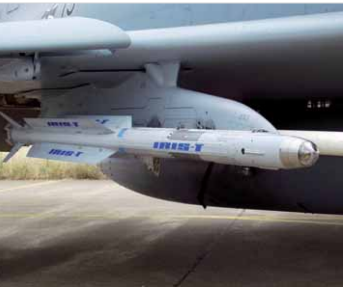
IRIS-T Guided Missile Mounted on a German EUROFIGHTER. Photo: Diehl
