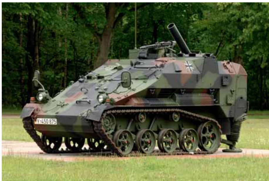
Air transportable light 120mm self-propelled mortar on WIESEL 2 chassis is the weapon carrier and thus the centerpiece of the mortar combat system consisting of different vehicle systems. Photo: Rheinmetall Defence
