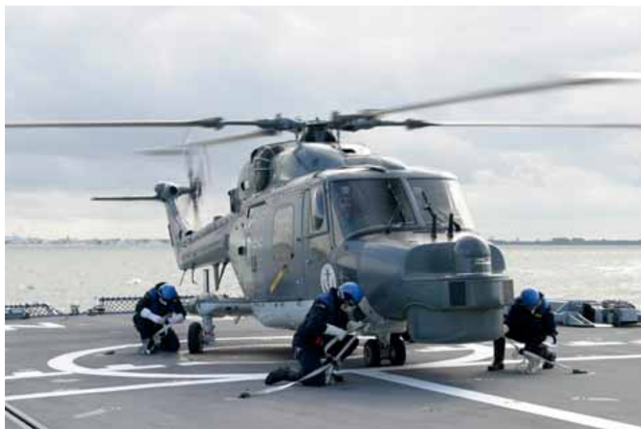
SEA LYNX Mk 88 Helicopter Being Fixed Aboard Ship after Landing.
