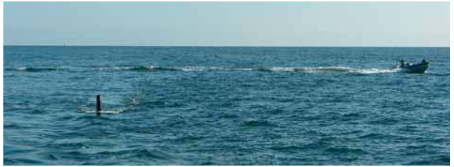
CALLISTO signal buoy has low, non-acoustic signatures. When additionally equipped with organic sensors, this system allows broadband communications from the depth with concomitant surveillance of the close-in area. Photo: Fa. Gabler
