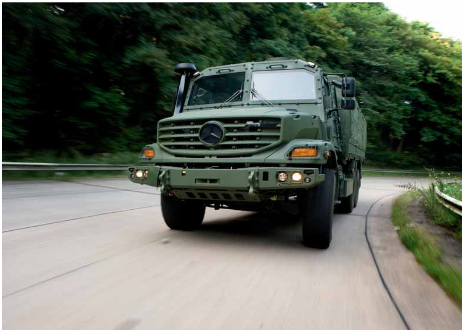
The 326 HP ZETROS 6x6 is a contender for the GTF 9t class.
