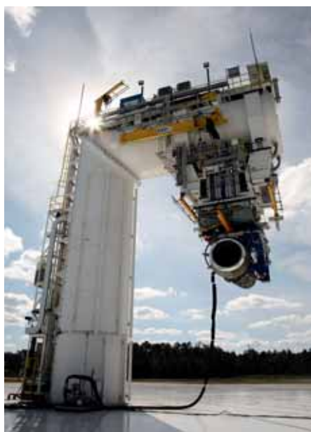
Testing of the BR725 engine at the Rolls-Royce outdoor jet engine testing facility, located at NASA's John C Stennis Space Centre, Mississippi, USA.
