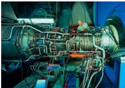
The German Navy's LM2500 industrial gas turbines are integrated by MTU Friedrichshafen GmbH and maintained by MTU Maintenance in the Berlin-Brandenburg plant. Picture: MTU Aero EnginesBerlin.
