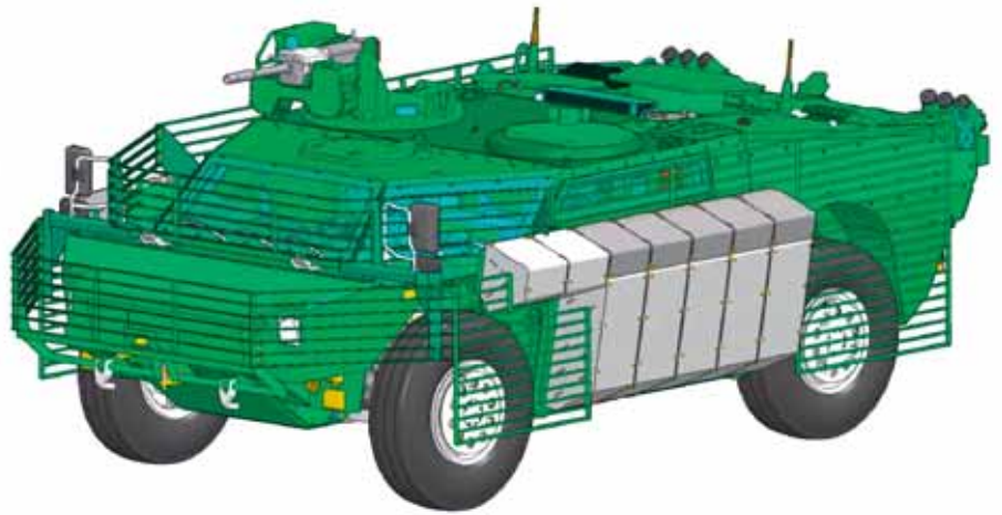
FENNEK reconnaissance vehicle with CLARA protective modules.
