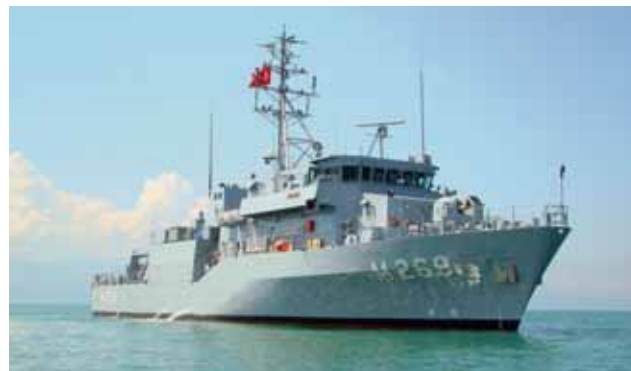
Mine Hunter made of Nonmagnetic Steel.
