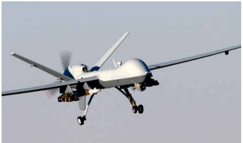
A MQ-9 Reaper UAV of the US armed forces in a landing approach after a mission in Afghanistan as part of Operation Enduring Freedom; the UAV can be equipped with precision bombs and air-to-ground guided missiles. Picture: Pentagon
