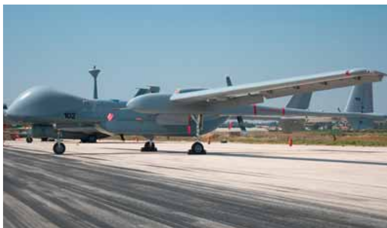
HERON is a very quiet, high-altitude, all weather-capable reconnaissance drone of the Israeli Air Force. It was developed by Israel Aircraft Industries (IAI) and is officially in service since early 2007. Its navigation is effected by an integrate GPS system. Launch, employment and landing happen fully automatically. HERON TP – also designated HERON 2 – is an advanced version of HERON 1. The PT6 turboprop engine provides HERON TP with a longer range, longer time on task, higher altitude and a four times heavier useful load.
