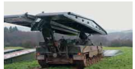
The LEGUAN bridge-layer on LEOPARD 2 chassis.
