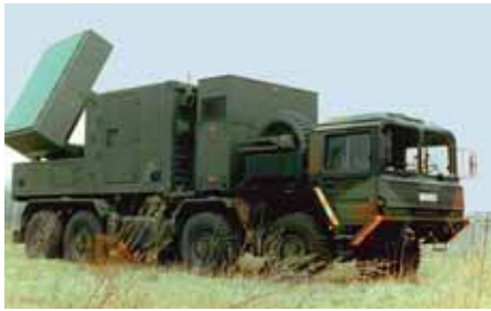
COBRA system of the German Army on MAN 8 x 8 truck. Picture: EADS
