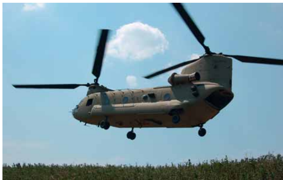
Boeing's CH-47F Helicopter can carry a Payload of nearly 10,000 kg. 48 Units are in Service with the U.S. Army since August 2008. Picture: U.S. Army
