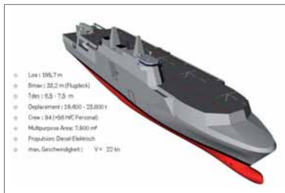
Figure 13 MEKO™ MESHHD — Main Dimensions.
