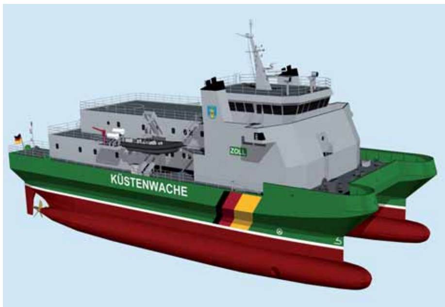
Figure 3 SWATH under Construction with TKMS for Use with German Customs Police.
